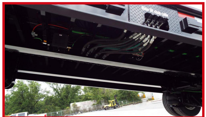
HYDRAULIC HOSES THREADED THROUGH MAIN BEAM WITH GROMMETS - STANDARD
